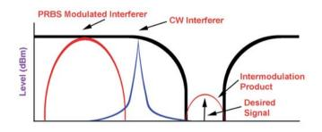
Figure 2 - Intermodulation Blocking Test
