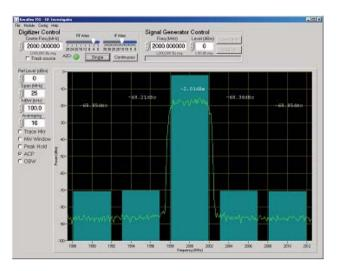
Figure 6 - Typical ACP Response of PXI Digitizers (3gpp, TM1, 64ch)
