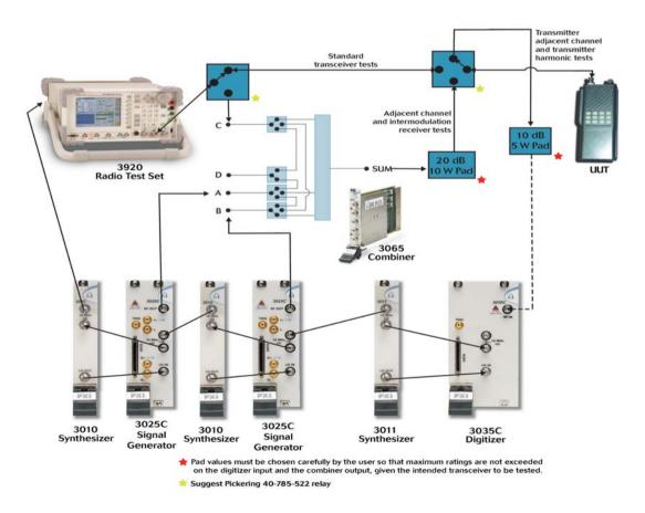
Figure 1 - Radio Conformance Interconnect Using 3920 and PXI
