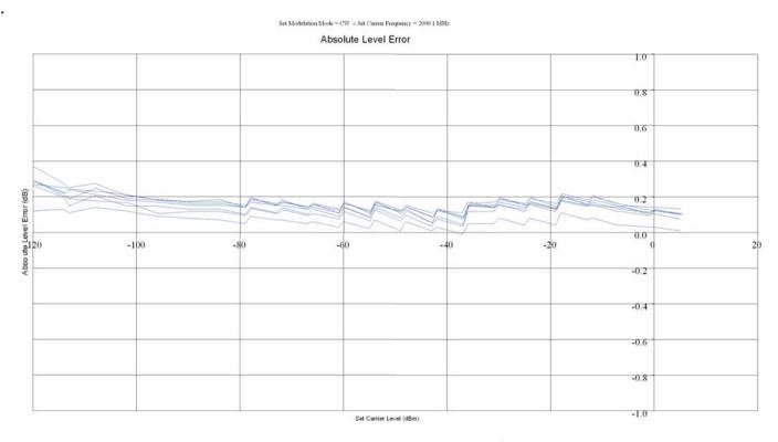
Figure 5 - Typical Level Repeatability of PXI Signal Generators
