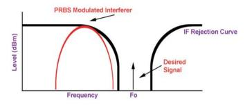
Figure 3 - Adjacent Channel Test
