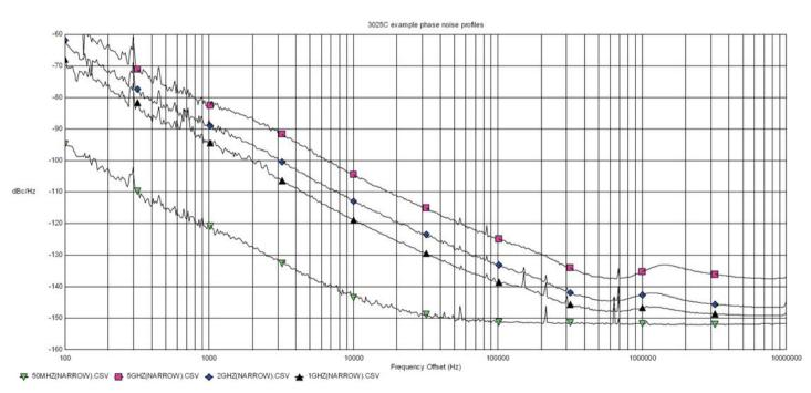
Figure 4 - Typical SSB Phase Noise Performance of PXI Signal Generators
