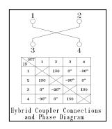
Mid-Atlantic RF Systems offers an extremely low loss 90 degree hybrid coupler operating at a nominal center frequency of 667 MHz. This is a high performance precision stripline hybrid which will handle up to 250 watts of CW RF power. This part is designed to directly replace the SAGE Wireline (0.25 inch square) with significant cost reduction without sacrificing performance.
