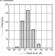
Measuring conditions Sample: CR2-12 V, 50 pcs. Equipment setting: "A" weighted, Fast, Max. hold Coil voltage: 12V DC Coil connection device: Diode Background noise: Approx. 20dB
