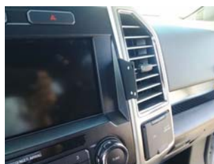
Bottom Part Installed
