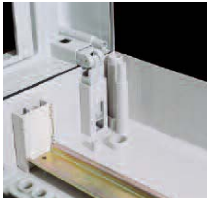
Hinges: should be snap-fitted into their guides, can be mounted on the left or the right side, in the series versions 12 to 64 DIN modules.
