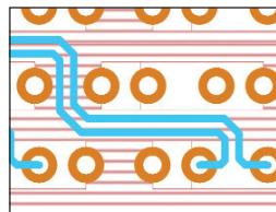
**Double ground vias are spaced 1.56mm apart providing a wide secondary routing channel.**
