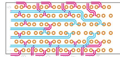
**Routing a 4-pair in two layers. First layer shown in blue, second layer shown in red.**
