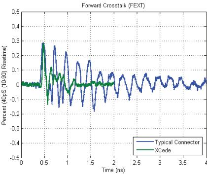
Use of advanced engineering materials in the shield eliminate crosstalk resonances, which appear as ringing through multiple bit periods in time-domain based measurements.
