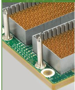
Amphenol's Xcede® connector platform is designed to enable future data rate requirements of datacom, telecom, storage and wireless equipment:
