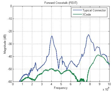
A unique 3-D resonance damping shield enables very low crosstalk across a wide frequency spectrum.
