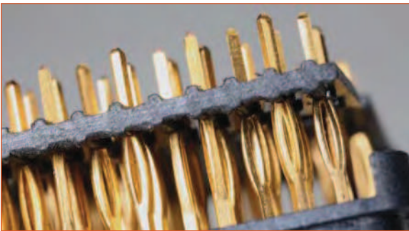
LRM backplane insert with compliant pins
