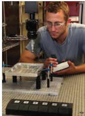
CMM measuring is done to check machined parts.
