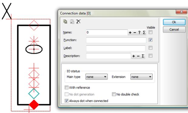
Dots for bridge connections will now be showed in graphical terminal plans.
