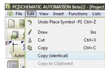
The function is only possible when you mark a symbol, and when this symbol is not a relay.
