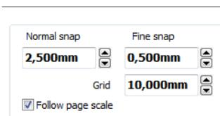
Normally, when you make mechanical drawings you work with fixed module sizes, and you wish to work with those sizes independently of the actual page scale. Now it is possible to have work with fixed module sizes and "jump" one module at the time.
