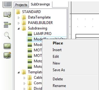
The button for inserting sub drawings in the Area toolbar is deleted and replaced by a new menu item "Insert" in the rightclick menu of the pathfinder window. The function of the menu item is equal to Ctrl-clicking or dragging.
