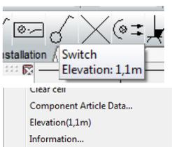
You can add elevation directly in the pick menu. If you have to symbols/components that are always placed in the same elevation the elevation can be added as a property to the symbol. If you need
