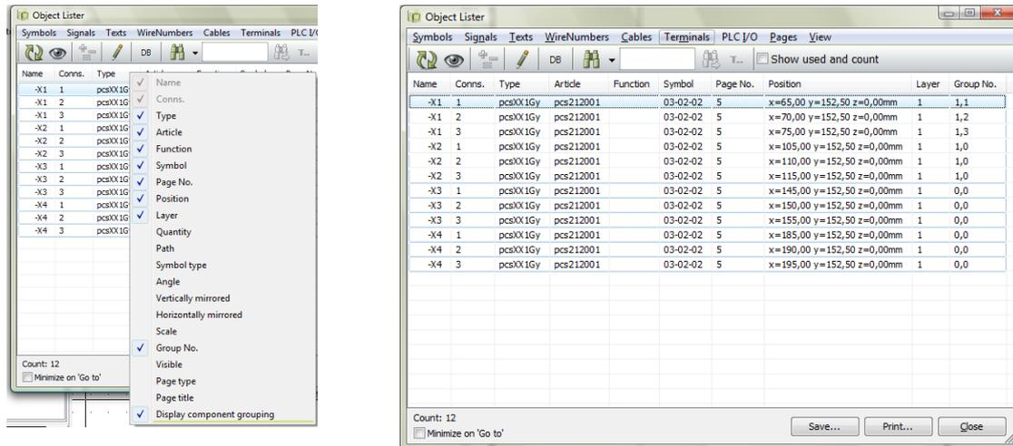
A more graphical edition of F7 has been made, and that should made component grouping more intuitive. Component grouping can be a very time consuming task, especially if you need to switch many some relations in the terminal row.
