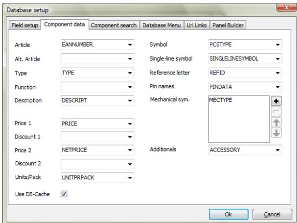
In order to make it possible to generate single line diagrams, the database must contain a single line symbol for each included component's power part.
