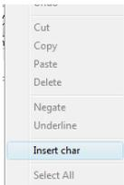
Inserting special characters by means of the Alt-button has been changed, as this cannot work together with the Unicode character sets. When you need to insert a special character in a text you right-click in the text window, and get the option "Insert char".
