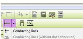
On mechanical pages you need to draw lines on top of lines on installation drawings, particularly when drawing "cables" instead of "lines". In order to avoid dots where there are no connections but only parallel cables, choose the lines without dot connection.
