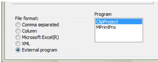
When you want to print labels for terminals, cables or other components, this is done with the "List to file" function. This has been extended (when the module is installed), making it possible to export directly to M-Print PRO.
