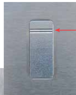
Depending on placement of the fastener within the mounting hole, a slight gap may be noticeable along the non-clinching edges of the fastener after installation.
