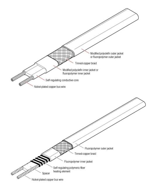
**Power-Limiting Heating Cables:** Power-limiting heating cables are the preferred technology for applications requiring high power output at elevated temperatures. These cables can be used for high maintain temperatures ranging up to 455°F (235°C) depending on cable selection and exposure temperatures to 482°F (250°C).
