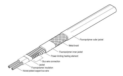
The positive temperature coefficient (PTC) of the heating element reduces power output as ambient temperature increases. This effect allows the power-limiting cable to be crossed over itself since the temperature of the heating element is reduced at the cross over points.
