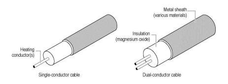
MI heating cable sets are supplied factory terminated and ready to install. They include a heating section and a cold lead (nonheating) section.
