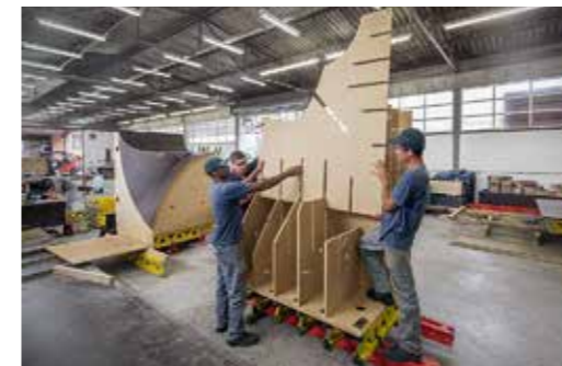
At the PERI facility in São Paulo, over 3,500 formwork elements were accurately manufactured in very high quality.
