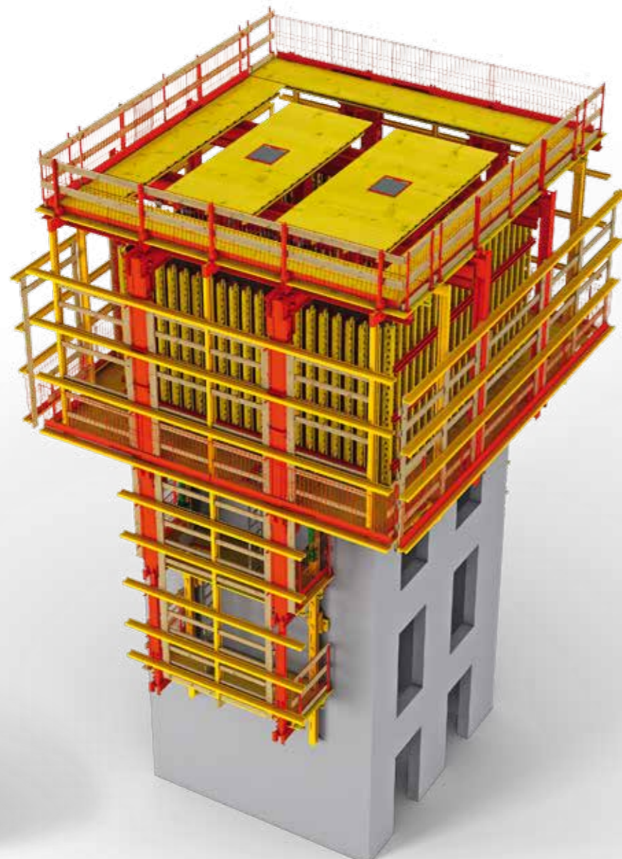
ACS P – the solution for advancing cores of high-rise buildings and tower-like structures – combined with ACS G. Both formwork sides are movably attached to the cantilevered platform beams.
