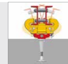
The RCS Climbing Rail can be inclined 4° in forward as well as reverse directions in order to climb over wall offsets.
