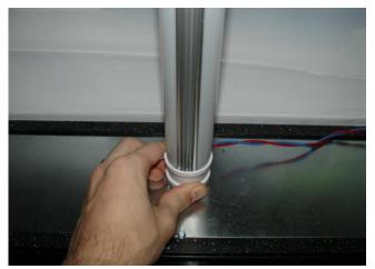
\*Note: For 8ft and 10ft Linearray<sup>™</sup> units, please ensure that the lamp holder plungers are spring-loaded only at the top
