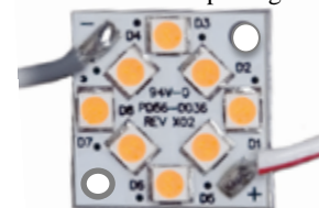
LED module with MCPCB and 3mm LED packages
