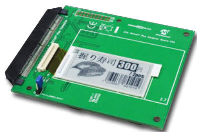
The EPD PICtail™ Plus Daughter Board assists with the development of electronic paper displays (EPDs).
