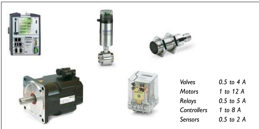
Typical nominal currents of electrical loads
