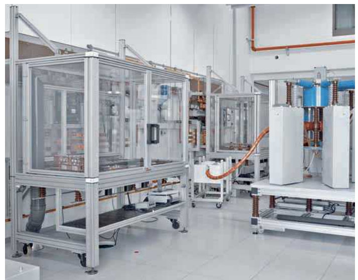
Fig. 24: Testing stations of the high-current testing system
