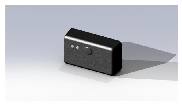
The Wi-Light dongle is a self contained wireless transceiver which can be added to any DMX controlled Photon Beard Hilight fixture. It outputs data directly into the DMX decoder and completely removes the need for any control cable. DMX cable may still be connected but priority is given to the wireless connection. The local manual fader and address setting will continue to work as normal.
