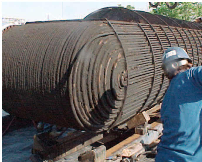
Oil cooler found at Strategic Petroleum Reserve is used to cool crude oil as it is extracted from the storage caverns. Photo courtesy of Sandia National Laboratories.
