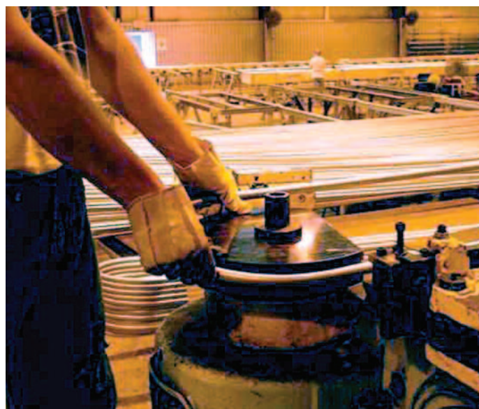
U-bending process of SEA-CURE® tubing supplied for the Strategic Petroleum Reserve oil cooler application. Photo courtesy of Plymouth Tube Co.
