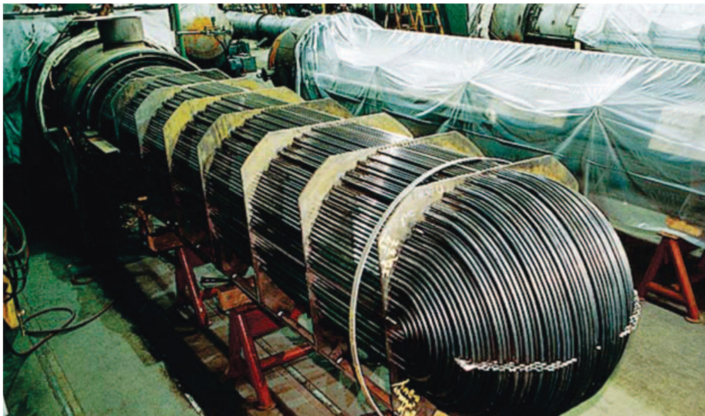
Plymouth Tube Co. supplied the chosen replacement tubing material SEA-CURE® for use in the Strategic Petroleum Reserve's heat exchangers.
