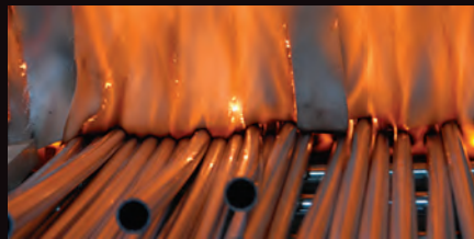
Tubing is heat treated in our bright annealing furnace to provide superior surface finish by eliminating scaling and surface imperfections.
