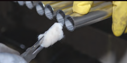
To ensure clean and dry tubing, tubing is handled by gloved technicians with the process of blowing felt plugs through the inside diameter of each tube.
