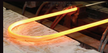
U-Bend tubing during the stress relieving process. Our XtraLowStress tubing offers the lowest possible residual stress in the industry.
