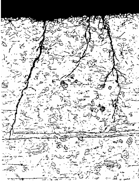
Figure 2 Transgranular Cracking in TP 304N Feedwater Heater Tubing
