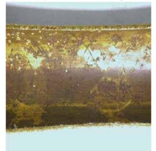
2. Copper alloys in condenser tubes often experience ammonia stress corrosion cracking and grooving. On the cooling water side, these same tubes experience erosion and corrosion when water velocities exceed 6 fps and pitting and under deposit corrosion. Courtesy: Plymouth Tube
