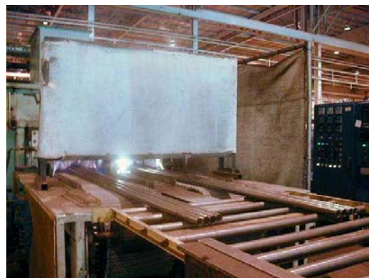
Figure 11 – Off-line furnace annealing of feedwater heater tubing
