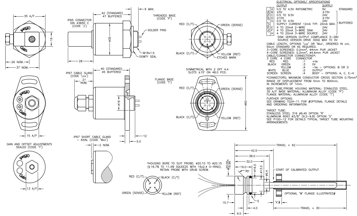
CONNECTIONS BETWEEN PROBE AND ELECTRONICS MODULE: FOUR WIRES; RED, BLACK, GREEN AND YELLOW, LENGTH: 300, CROSS SECTION: 0.25mm2, WIRES POTTED IN PROBE HOUSING. INTERCONNECTIONS MUST BE PROTECTED FROM WATER INGRESS AND STRAIN RELIVED.
