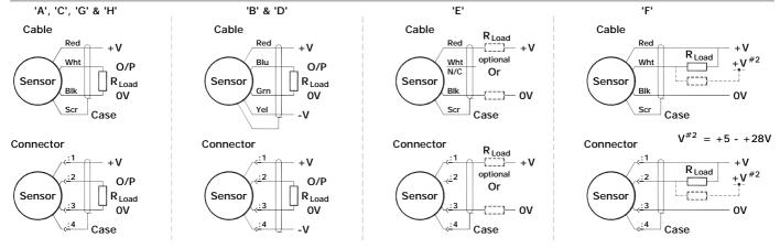
N.b. Sensors with options Ixx, Lxx or Mxx supplied with; 3-core cable: output options A, C, E, F-H, 4-core cable: output options B or D.
