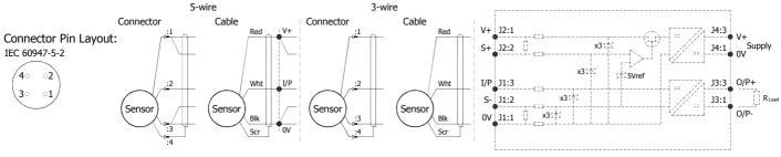
**Putting Into Service:** The sensor must be used with a galvanic isolation barrier designed to supply the sensor with a nominal 5V and to transmit the sensor output to a safe area. The barrier parameters must not exceed:-
