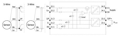
**Putting Into Service:** The sensor must be used with a galvanic isolation barrier designed to supply the sensor with a nominal 5V and to transmit the sensor output to a safe area. The barrier parameters must not exceed:-
