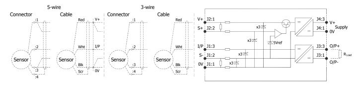
To ensure correct operation of both Amplifier and sensor, the following restrictions on conductor cross section and cable length limits are set out below (figures are based on copper conductors);
