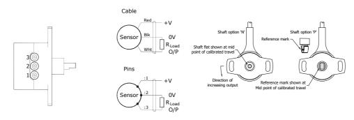
**Mechanical Mounting:** Flange mounted. The flange slots are 4.5mm by 20 degrees wide, 48mm pitch. The sensor should be mounted with minimal axial and radial loading on the shaft for optimum life. It is recommended that the shaft is coupled to the drive using a flexible coupling.
