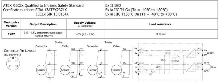
**Putting Into Service:** The sensor must be used with a galvanic isolation barrier designed to supply the sensor with a nominal 5V and to transmit the sensor output to a safe area. The barrier parameters must not exceed:-
