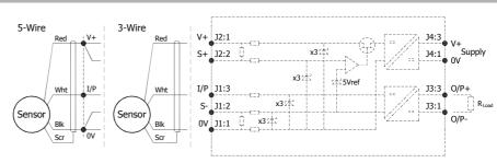
**Putting Into Service:** The sensor must be used with a galvanic isolation barrier designed to supply the sensor with a nominal 5V and to transmit the sensor output to a safe area. The barrier parameters must not exceed:-
