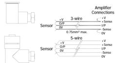
For this reason Positek® recommends five wire connections for cable lengths exceeding 10 metres in 0.25 mm² cable to preserve the full accuracy of the sensor.
