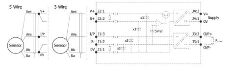
**Putting Into Service:** The sensor must be used with a galvanic isolation barrier designed to supply the sensor with a nominal 5V and to transmit the sensor output to a safe area. The barrier parameters must not exceed:-
