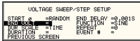
Figure 4-13: VOLTAGE SWEEP/STEP SETUP Screen
