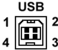
Figure 3-11: USB Connector pin orientation.
