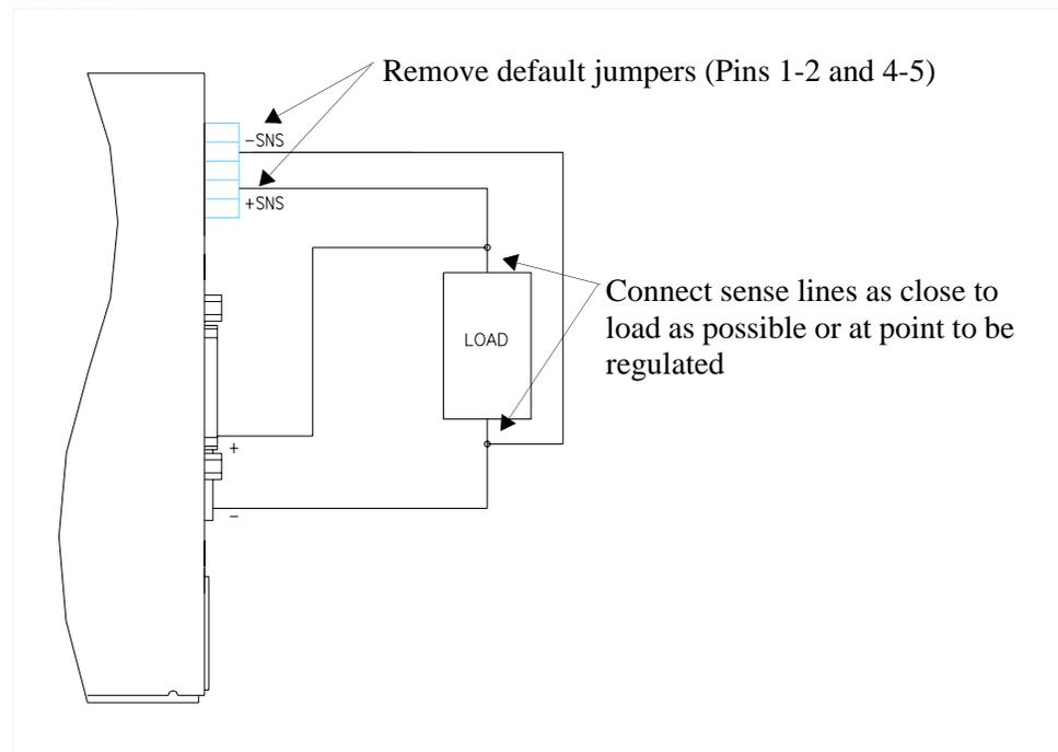
In order to connect the sense wires, follow this procedure:
