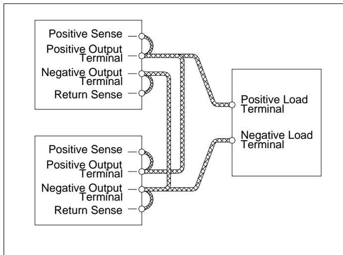
**Figure 3.3** Parallel Operation
