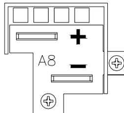
**Figure 1.4** Output Busbars - note polarity markings
