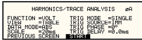
Figure 3-16: HARMONICS/TRACE ANALYSIS screen
