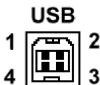
Figure 3-4: USB Connector pin orientation.
