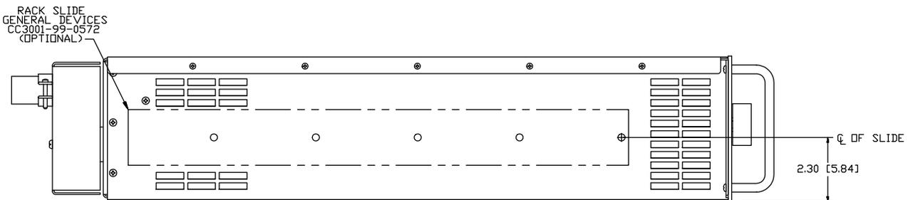
Figure 8-1: Rack Mount Slides (-RMS option) position
