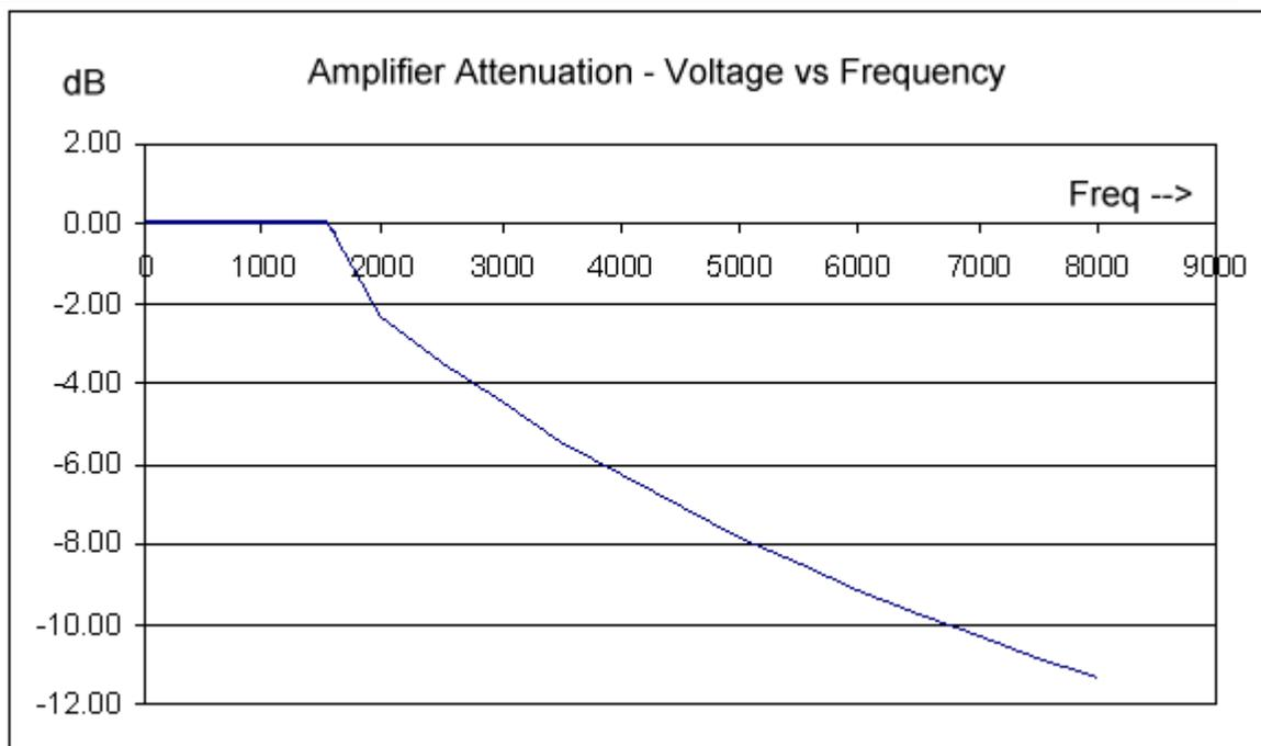
Figure 2-8: Typical frequency response, low Vrange, ALC off.
