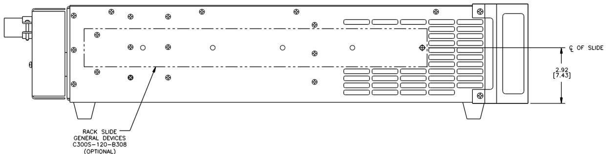
Figure 2-2: Rack Mount Slides (-RMS option) position
