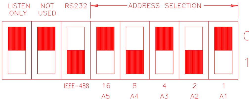
Figure 8-2: GPIB Address Selection Switch
