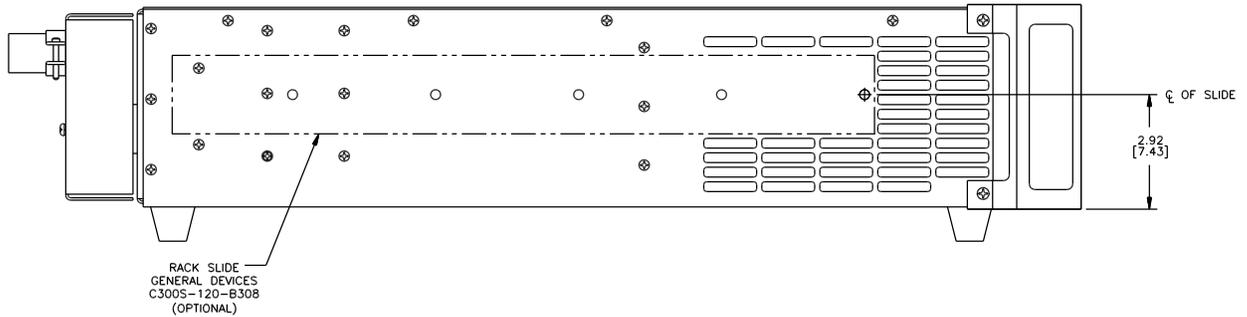
Figure 3-5: Rack Mount Slides (-RMS option) position
