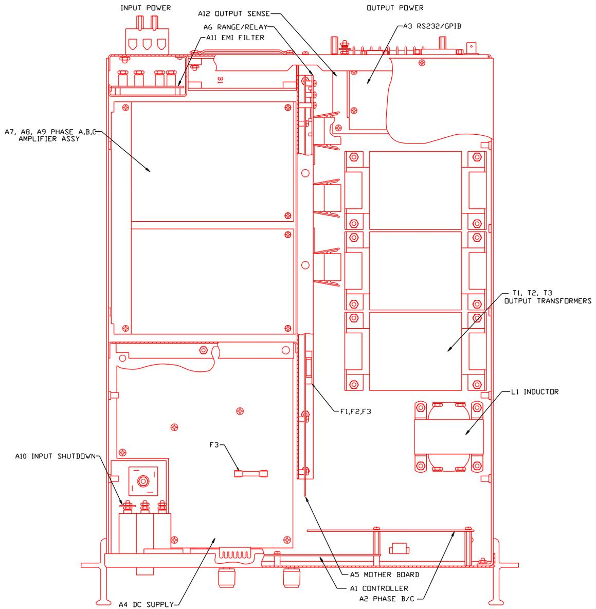
Figure 7-1: Assembly Location
