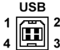
Figure 3-11: USB Connector pin orientation.
