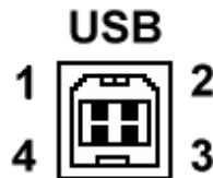
Figure 3-16: USB Connector pin orientation.
