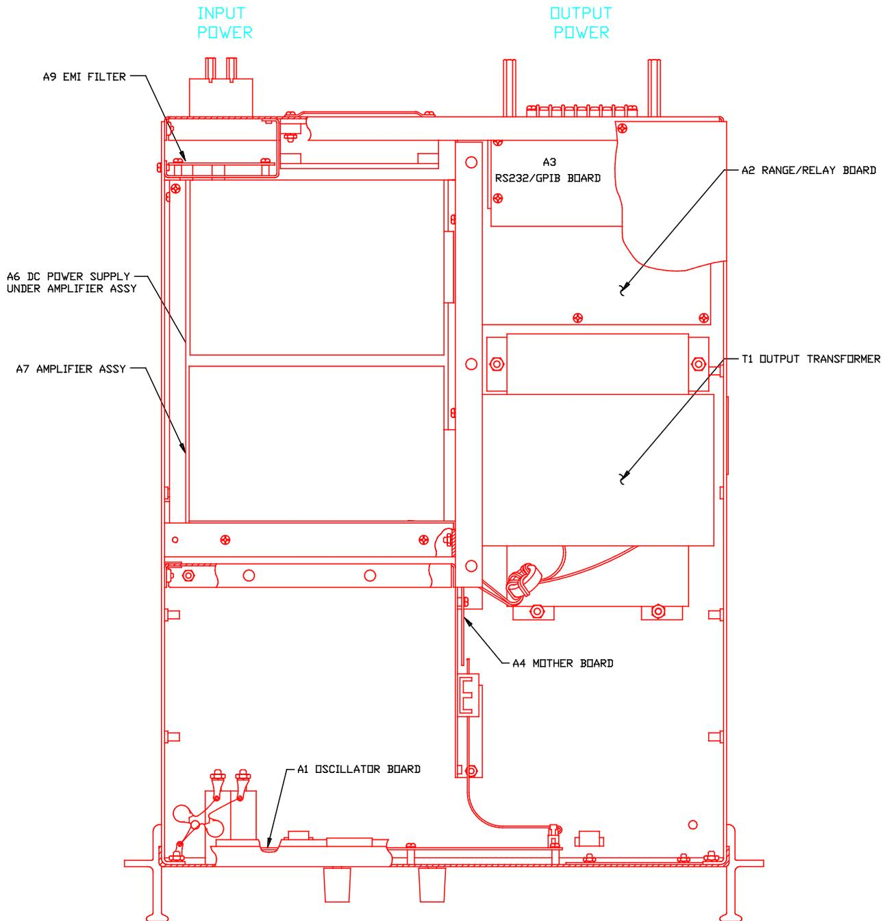
Figure 7-1: Assembly Location
