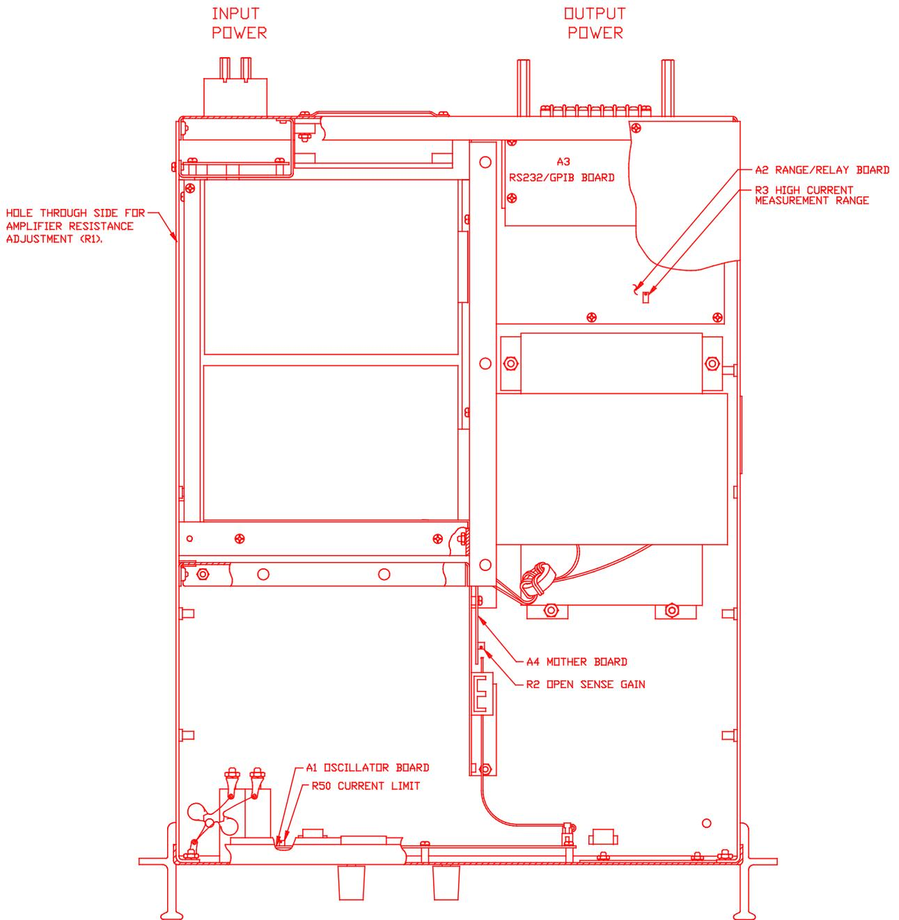
Figure 6-3: Internal Adjustments
