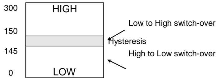
Figure 4-2: Voltage Auto Range Switch Over Points
