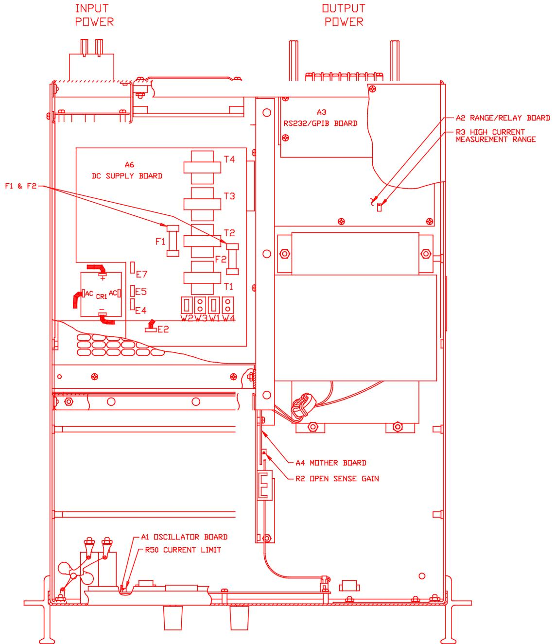
Figure 3-3: Internal Adjustments and Jumper Locations, Input Line Voltage 103 to 127
