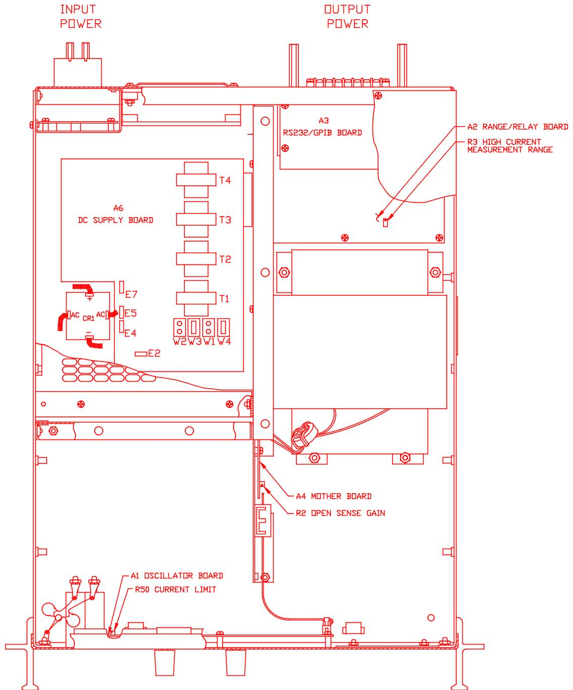
Figure 3-4: Internal Adjustments and Jumper Locations, Line Voltage 187 to 253 Volts
