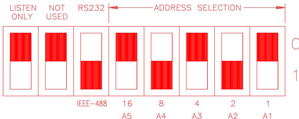
Figure 8-2: GPIB Address Selection Switch
