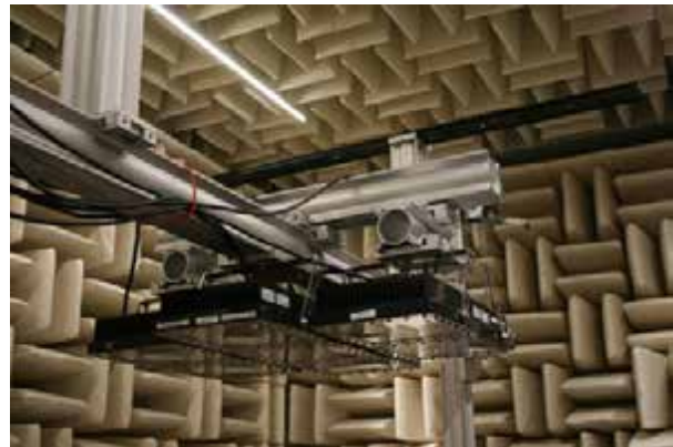
Fig. 4: Horizontal and vertical construction using X 95 and Flat Rail components for research applications.
