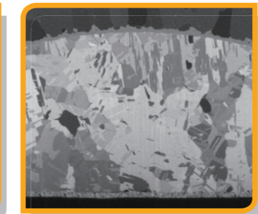
Bump Grain Orientation_Dual FIB
