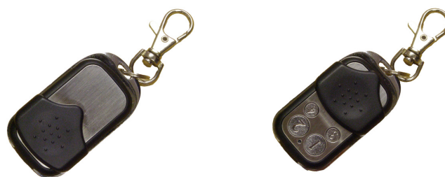
Transmitter Showing Sliding Cover
