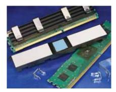
Gap Pad HC 1000 is an extremely conformable, low-modulus polymer that acts as a thermal interface and electrical insulator between electronic components and heat sinks. The "gel-like" modulus allows this material to fill air gaps to enhance the thermal performance of electronic systems. Gap Pad HC1000 is offered with removable protective liners on both sides of the material.
