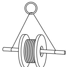
Reels can be hoisted with a properly secured shaft extending through both flanges.
