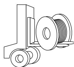
Never allow fork tines to touch the cable surface or reel wrap.
