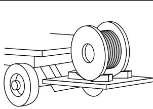
Lower reels from a truck using a hydraulic gate, hoist or fork lift.
