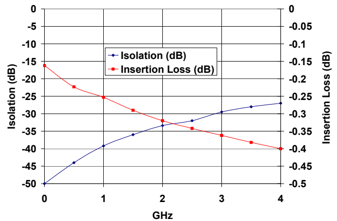
Fig. 5. Capped switch isolation and insertion loss vs. frequency for a 4-contact microswitch.
