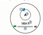
The destination indicator ① shows the direction of your destination relative to the direction you are moving ②. When the destination indicator appears at the top of the circle, you are heading toward your destination. The remaining distance to your destination ③ appears below the circle. The progress bar ④ shows your progress toward your destination.
