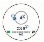
The destination indicator ① shows the direction of your destination relative to the direction you are moving ②. When the destination indicator appears at the top of the circle, you
