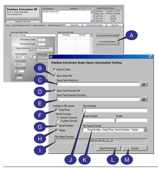
The Production Testing Mode enables the user to quickly test multiple components and save the results to a file in an automated fashion.
