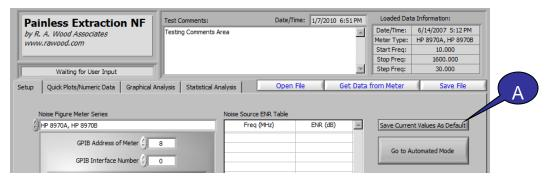
Painless Extraction NF utilizes a settings file to store the default test setup that is loaded at the start of program operation. This file is stored in an \*.ini format. The following parameters are saved in the default setup file:
