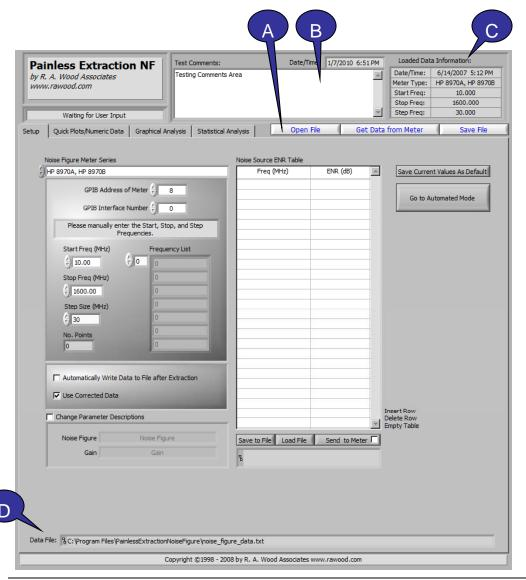
The Setup Tab is primarily used at the start up of the program. On this tab you will find all the parameters necessary to import a data file or to extract data from a noise figure meter.
