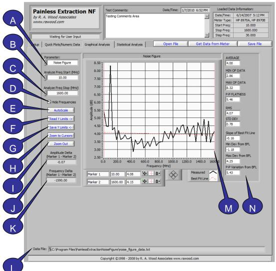
The Graphical Analysis Tab provides a large plot of the selected parameter and detailed statistical analysis.
