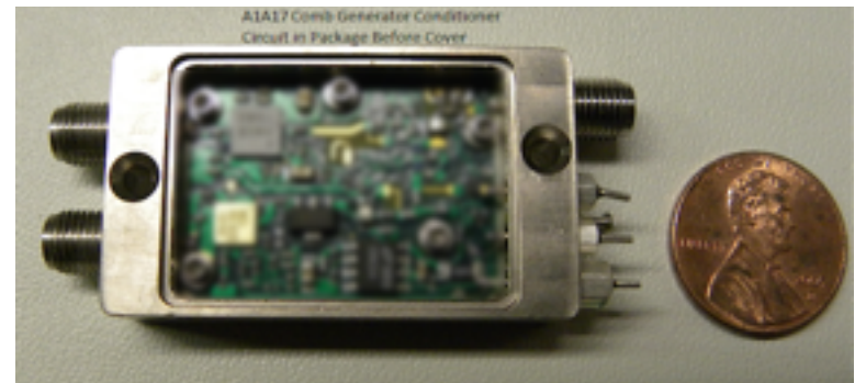
A1A17 RF SubAssembly provides LO signals up to 15 GHz
