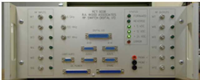
Custom designed Test Interface Box
