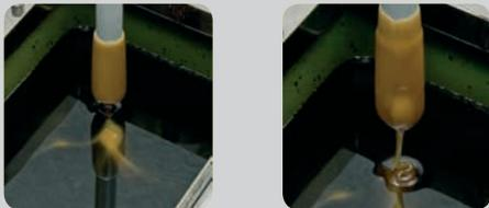
The probe also switch off reliably even if there is still a glue thread connection between probe and the residual glue at the bottom of the empty container.
