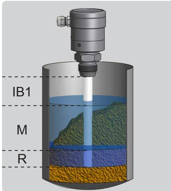
On the left you see a schematic drawing of the measuring ranges of a filling level probe with two measuring points. You see, that the probe measures a range that is like a disc and not just a small area around the probe.
