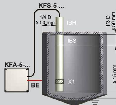
The probe can be mounted centrally or eccentrically. For a measurement independent of the filling cone, we recommend that the probe be mounted at a 1/4 of the diameter. The minimum distance between the upper switching point and the conductive lid of the container is 50 mm.
