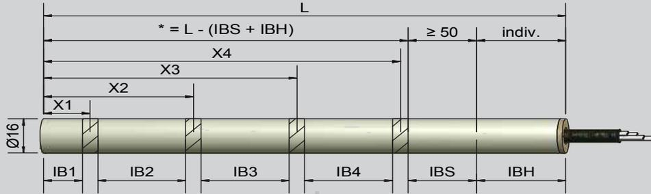
The limit probe can be equipped with one, two, three or four fixed switching points.
