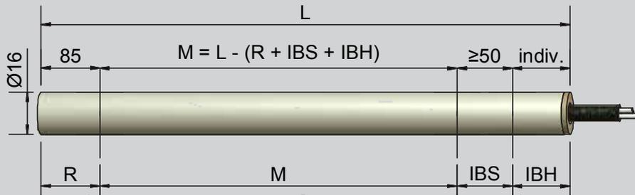
The **analogue probe** consists of a **reference system (R)** at the top of the probe to determine the existing material characteristics. This reference range stretches over 85 mm independent of type.
