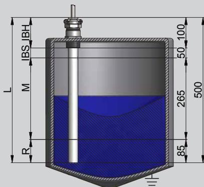
Example for a probe with PTFE body and a total length of  $L = 500 \text{ mm}$  with a holder ((Art. Nr. 194 000)  $IBH = 100 \text{ mm}$ ). For  $IBS$  the min. distance of 50 mm has been applied. This results in an available measuring range  $M = 265 \text{ mm}$ . The calculation is as follows:
