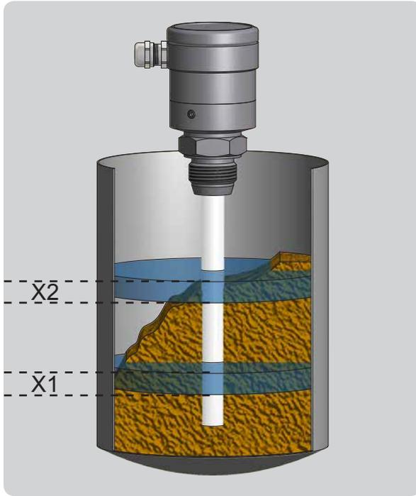
On the left you see a schematic drawing of the measuring ranges of a filling level probe with two measuring points. You see, that the probe measures a range that is like a disc and not just a small area around the probe.
